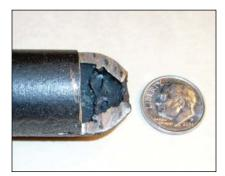
Fig. 2. Cut-away view of a ½-inch NPT, Inconel 601 protection tube welded closed with the wrong material.
