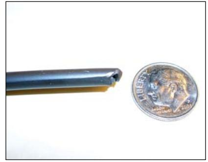
**Fig. 3. A blown-out or “popcorn” tip resulting from the wrong welding material and internal moisture.**
