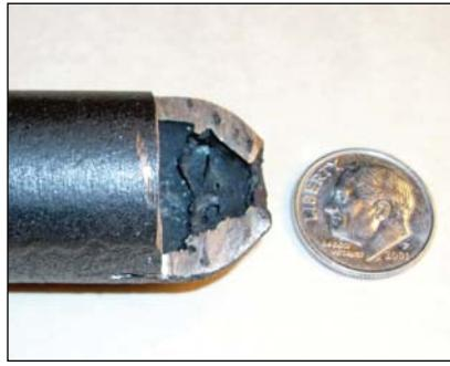
**Fig. 2. Cut-away view of a ½-inch NPT, Inconel 601 protection tube welded closed with the wrong material.**
